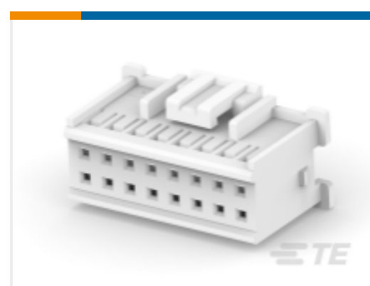
TE Part # 1-2323743-6 HOUSING, PLUG, GWT, 16P, DUAL ROW, EP2.5
